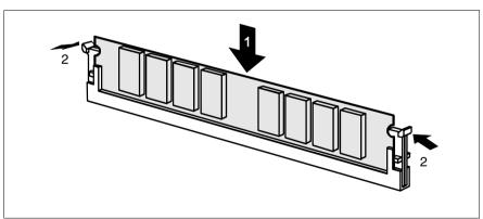
Figure 5: Installing a memory module
